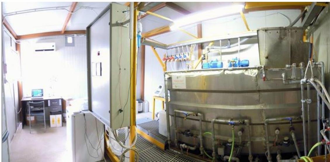
**Nitrogen removal pilot plant (Anammox battery experimentation working on sludge digestate)**
